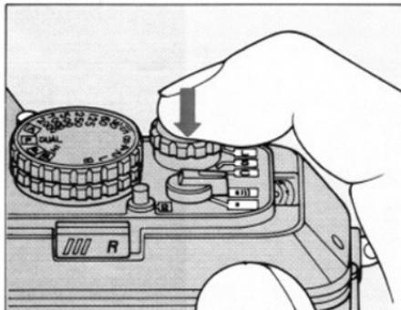
4. Confirm that the green in-focus indicator LED lights up, then fully depress the shutter release button to get a correctly focused image. Fully depressing the shutter release button with the green in-focus LED off may result in an out-of-focus image.
