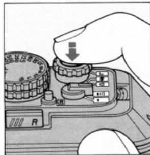
3. Lightly press the shutter release button to start the Continuous Servo Autofocus function.
