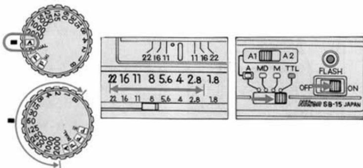
Select appropriate aperture. Set the N2020 to A or one of the manual settings. Determine aperture using the speedlight exposure calculator dial. (See flash unit instruction manual for details.) Set the speedlight mode selector to TTL and turn the speedlight on. Look inside the viewfinder and lightly press the shutter release button. When the ready-light comes on, you can shoot.
