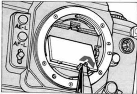
3. Remove the screen by grasping the small tab with the tweezers.
