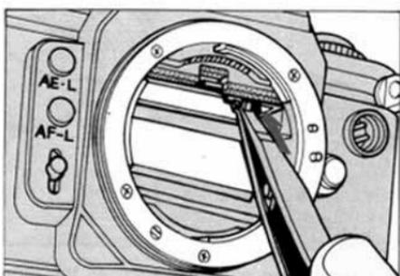
5. Using the tweezers, push the front edge of the holder upward until it clicks into place.
