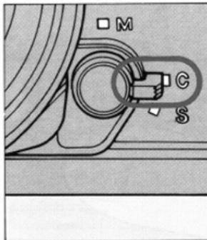
1. Set the focus mode selector to C for Continuous Servo Autofocus.
