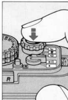
1. Center the focus brackets on the subject and lightly press the shutter release button.
