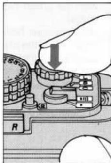
3. Keeping the shutter release button lightly pressed, recompose, then fully depress the shutter release button.
