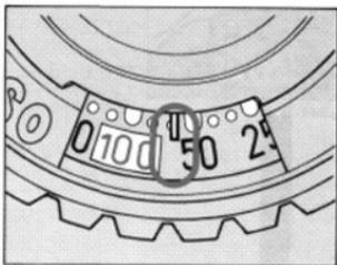
With non-DX-coded film, set to appropriate film speed.
