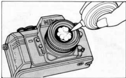
7. Clean glass surfaces such as the lens or the viewfinder eyepiece with a blower brush; avoid using lens tissue as much as possible. Wipe dirt and smudges, using soft cotton moistened with pure alcohol, in a spiral motion
