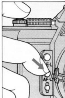
2. Keeping the shutter release button lightly pressed, confirm that the in-focus indicator LED lights up, then depress the AFL button and hold it in.
