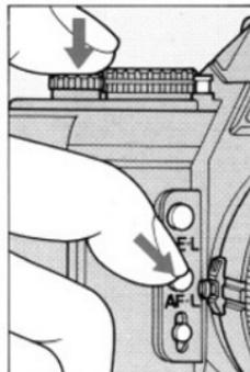
3. With the AFL button depressed, recompose as desired and fully depress the shutter release button.
