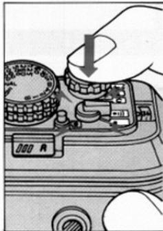
**22. Film winding stops automatically at end of film.**
