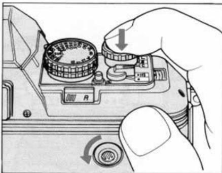
**15. Fully depress shutter release button to automatically advance film to frame "1."**
