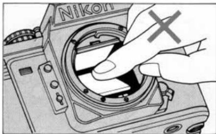
1. Never touch the reflex mirror and focusing screen. Remove dust with a blower brush.
