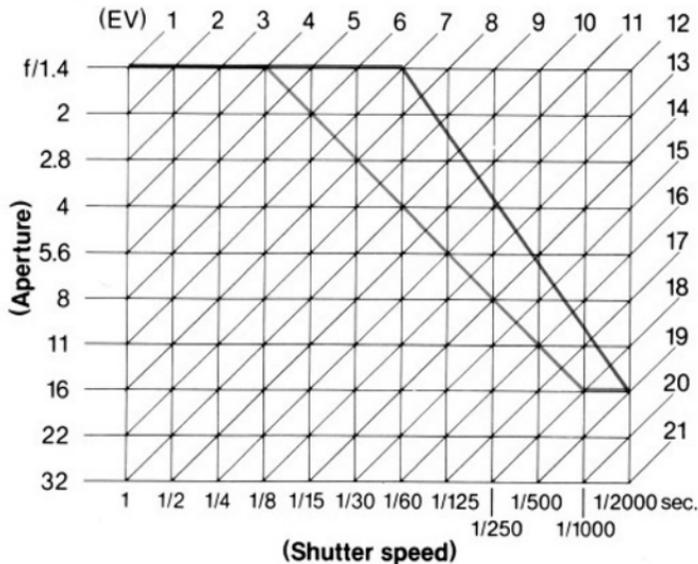
The EV (exposure value) chart demonstrates the difference between the N2020's normal and high-speed programs. Follow either colored line to where it intersects a diagonal line. This shows the combination of aperture (vertical line) and shutter speed (horizontal line). For example, at a brightness of EV12, the N2020 selects f/4 and 1/250 sec. at P HI; f/5.6 and 1/125 sec. at P (with 50mm f/1.4 lens at ISO 100).
