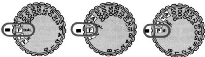
The N2020 microcomputer automatically sets the optimum combination of shutter speed and lens aperture. The N2020 offers three programmed automatic modes—dual, normal and high-speed—P DUAL for dual, P for normal, and P HI for high-speed.
