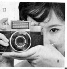
When holding the camera in the horizontal position, place your left hand under the camera, with your forefinger on the focusing lever of the lens (Fig. 17a). Grasp the camera with your right hand, cradling the lower right hand corner of the camera in the palm of your hand.
