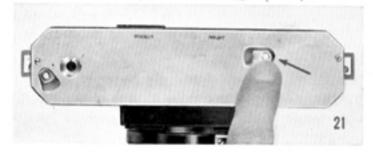
To rewind, first push in the rewind button (Fig. 21) found on the bottom of the camera (not the camera back release button), then lift the rewind crank (Fig. 22) and turn in the direction of the arrow. As the film is being rewound, a slight resistance will be felt and the depressed button on the
