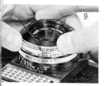
Holding the shutter speed ring turn the film speed ring found at the front end of the lens to bring the speed rating of the loaded film opposite the red index (Fig. 9). It can be set for either color or black-and-white film according to the film speed rating.
